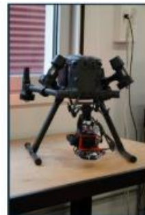
UAVs (drones) with cameras for blade surface monitoring
