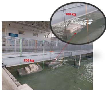
Concrete UHPC prototypes in floating tests with different loads
