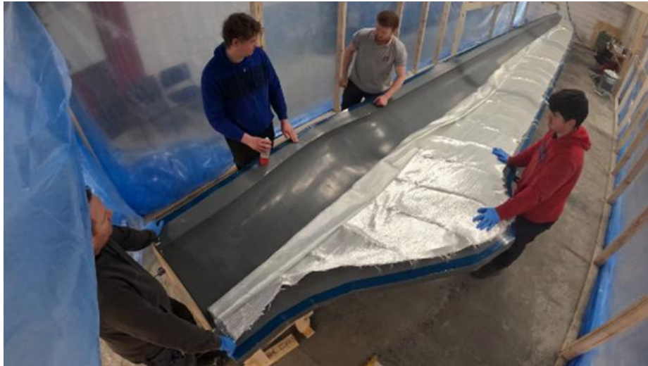
Successfully manufactured a 13-meter blade.
