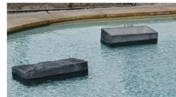
Buoyancy tests at lab scale for design purposes
