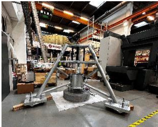
Coupons coated with antifouling (TECNAN) in GBS structure (INEGI)
