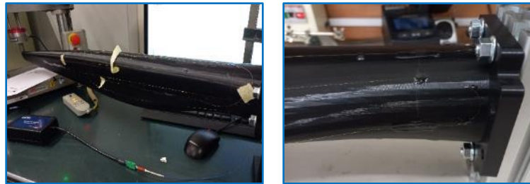
Scaled geometry SHM setup with FBG Strain gauge placement
