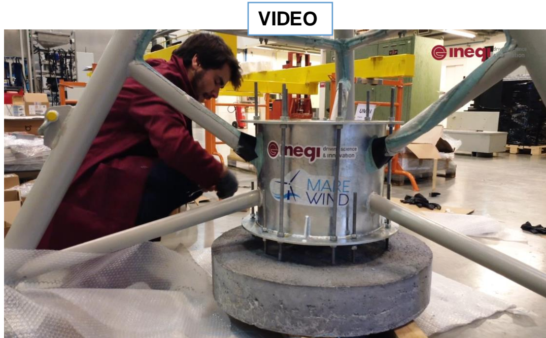
Coupons coated with antifouling (TECNAN) in GBS structure (INEGI)
