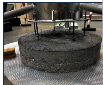
Alkali Activated Material concrete ballast specimen
