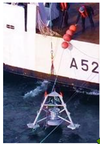
Alkali Activated Material concrete ballast specimen
