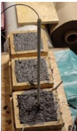
AAM concrete ballast Fiber Optic bars and sensors
