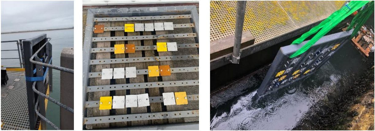
Tests conducted across atmospheric, splash zone, and subsea conditions
