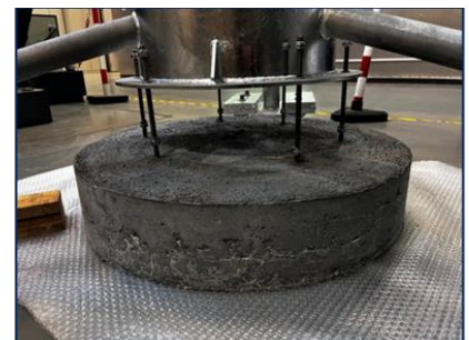
GBS in Sines (Portugal). Analysis after 6 months exposure in the GBS submerged in Sines
