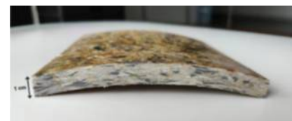
Material demonstrator of the novel composites recycling procedure developed by CETMA.
