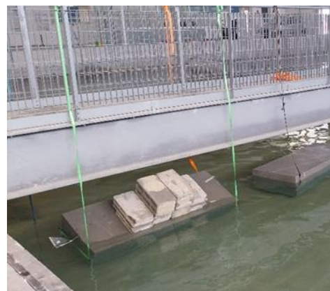
Wave basin for floating prototype testing (left image) and wave channel for gravity prototype testing (right image)
